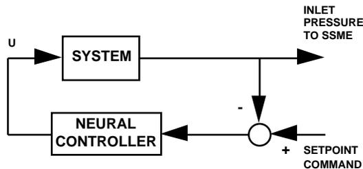
**Figure 2.2.** Simulation Scheme for NNC and System
