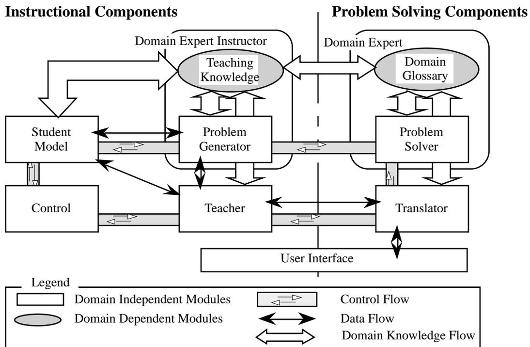
**Figure 1.** System architecture of I<sup>3</sup>'s intelligent teaching system
