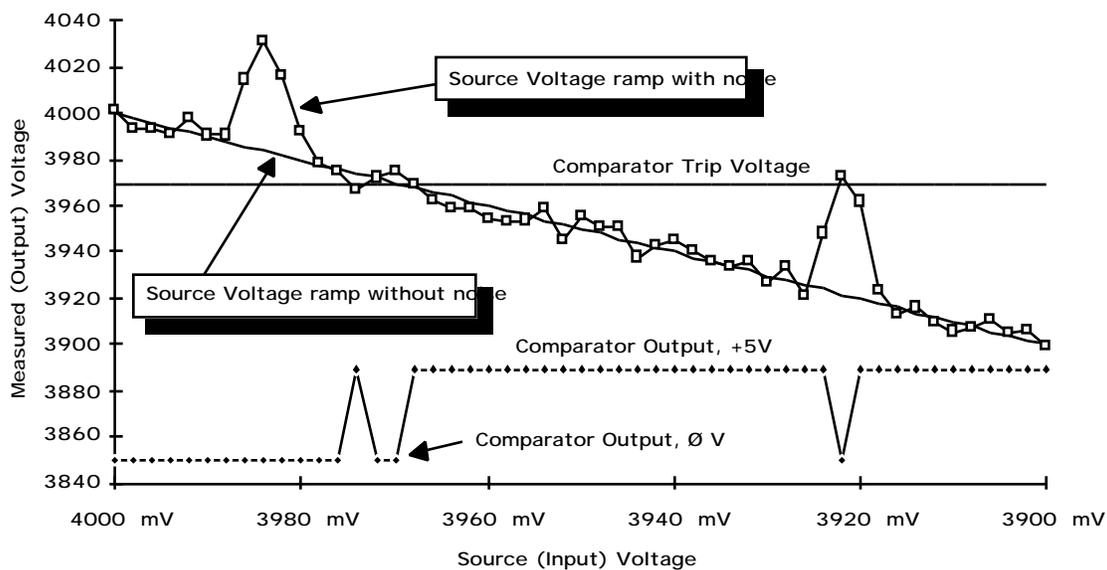
**Figure 3.** Noise Waveform During Test
