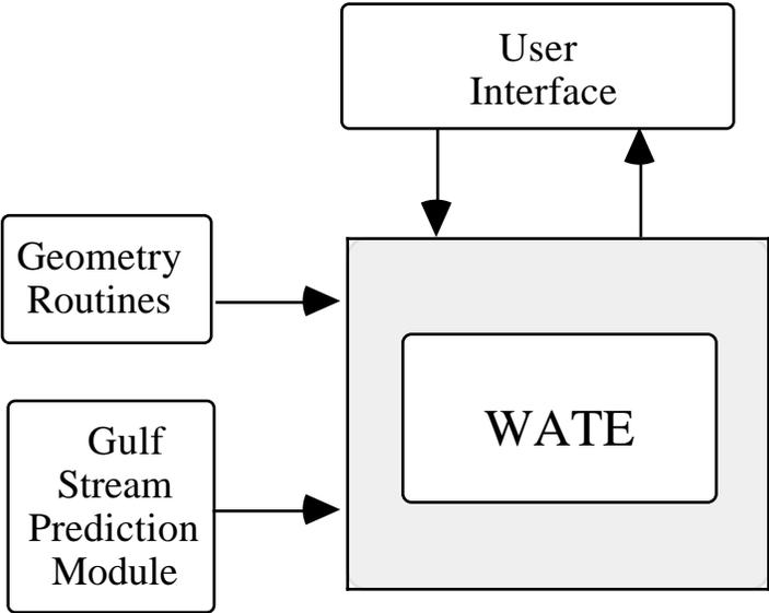
Figure 1. External Interfaces of WATE
