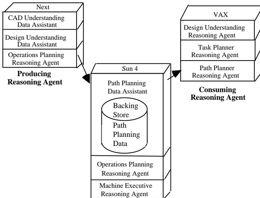
**Figure 1.** Architecture of the Distributed Artificial Intelligence Toolkit
